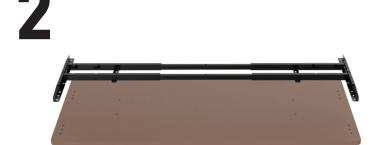
Place on the tabletop. Ensure that the correct side of this assembly is facing upwords.
